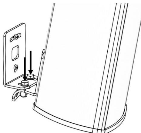
Adjust the speaker to the desired position by tilting and panning before tightening the screws highlighted above.
