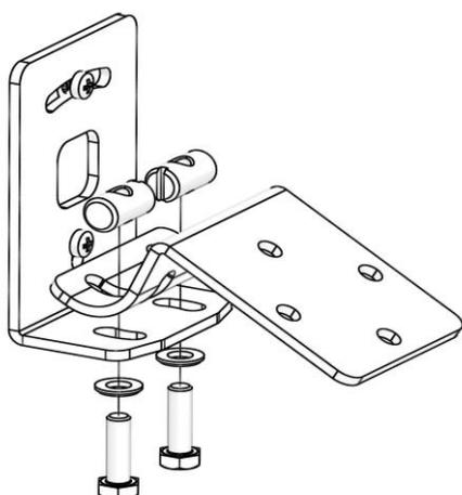
For mounting positions in the right-hand column of page 1, assemble the parts as shown above. Do not tighten the screws completely yet.
