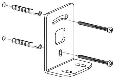
Mount the wall plate to the wall using suitable screws and dowels. (Screw diameter max. 5 mm)
