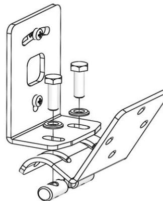
For mounting positions in the left-hand column of page 1, assemble the parts as shown above. Do not tighten the screws completely yet.
