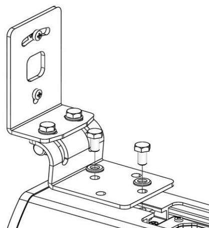
Position the housing plate anywhere along the T-slot of the cabinet. The slot nuts are supplied with the speaker.
