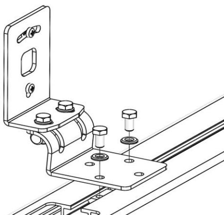
Position the housing plate at the centre of gravity of the cabinet. For speakers longer than 1.3 m we recommend using two WS-4 at a distance.
