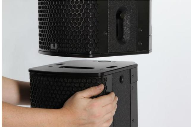
7. Carefully lower the suspended module until it sits on top of the standing module. Stop the motor as soon as the chain loses its tension. Then align both modules horizontally with one another.
