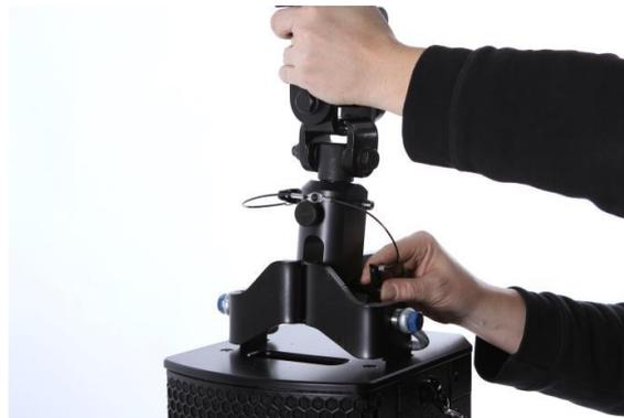
2. Lower the traverse or bar from which the system is to be flown until the CC-300's half coupler can be attached. Manually tighten the clamp in the first instance.
