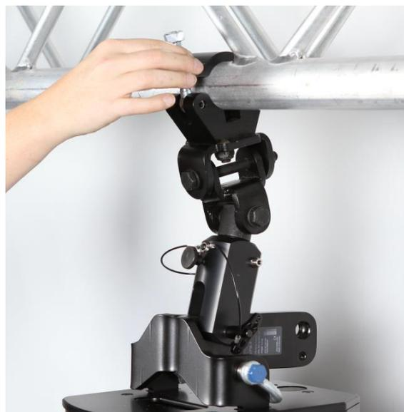
3. Raise the traverse until the first module is hanging freely above the floor. The CC-300 will have now aligned itself vertically. Then, tighten the nut of the half coupler firmly and secure it with the lock nut.
