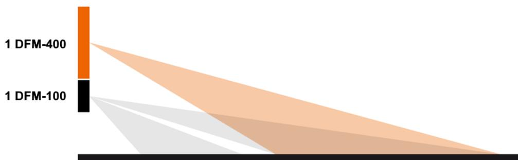
1b: 1x DFM-400 and 1x DFM-100 with a maximum room depth of 30 m. A second DFM-100 beam covers the nearfield area.
