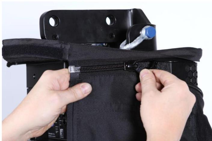
4. Close the rain cover by pulling the zipper that runs the length of its side. The remaining opening above the connector panel will then be covered by the two flaps. Stick the flaps together using the Velcro strips. Therefore, hold the flaps in place from the inside.
