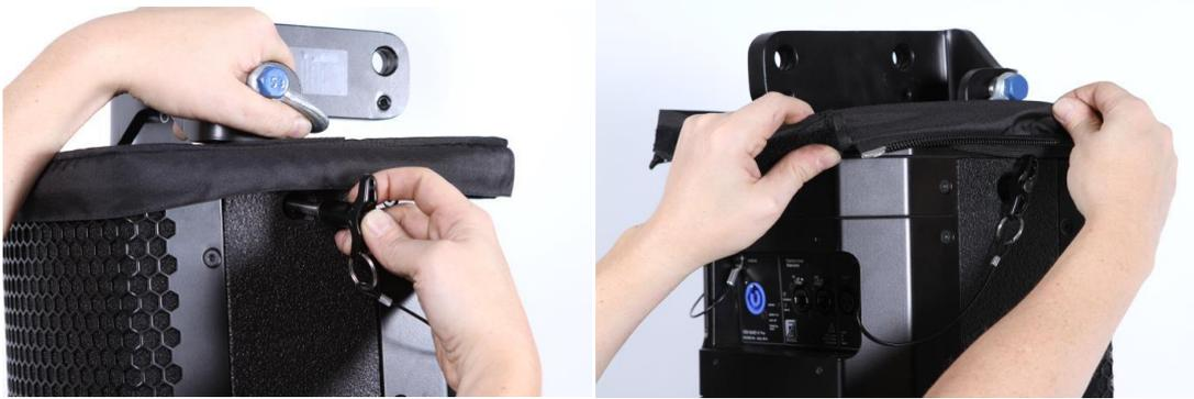
3. Join the lid with the covers' side elements using zippers. The actual positioning of the rain cover on the loudspeaker enclosure is determined by the sewn-in magnets, which adhere to the front grille. Move the magnets and pull the cover tightly forwards and downwards simultaneously.
