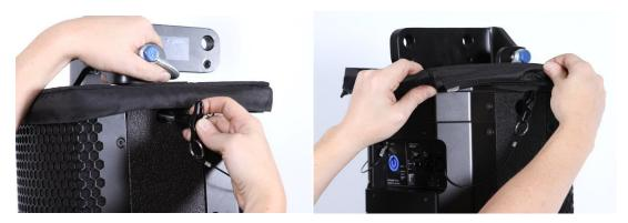
3. Join the lid with the covers' side elements using zippers. The actual positioning of the rain cover on the loudspeaker enclosure is determined by the sewn-in magnets, which adhere to the front grille. Move the magnets and pull the cover tightly forwards and downwards simultaneously.
