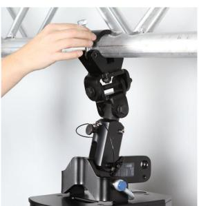
3. Raise the traverse until the first module is hanging freely above the floor. The CC-300 will have now aligned itself vertically. Then, tighten the nut of the half coupler firmly and secure it with the lock nut.
