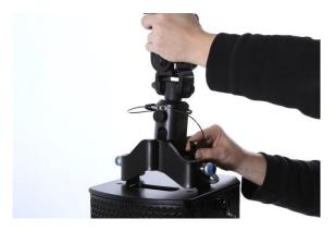
2. Lower the traverse or bar from which the system is to be flown until the CC-300's half coupler can be attached. Manually tighten the clamp in the first instance.
