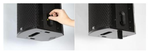
To connect the Focus Modular modules to one another, or to flying adapters, two ball lock pins are used. During transportation, these ball lock pins can be securely housed in two pilot holes on the connector panel.
