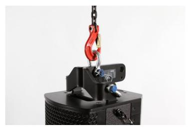
4. Fasten the safety bridle to both 1t shackles. If using separate cables or chains for both points, make sure that these are exactly of the same length and that they are attached to the same point. Please refer to section 3.2.4.
