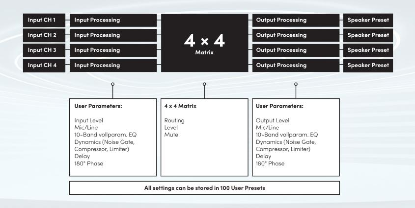
The integrated Fohhn DSP functions are easily controlled centrally via Fohhn Audio Soft. All tools can be applied to both input and output channels. Y ou can easily save your settings and presets - with password protection if required.
