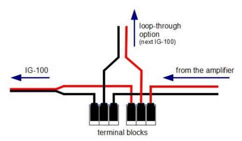
In the above diagram, the red cable represents the positive pole and the black the negative.
