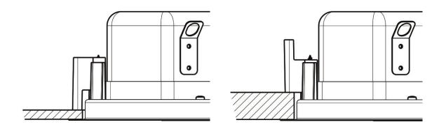
To rotate the mounting clamps for ceiling thicknesses of > 18.5 mm, proceed as follows:
