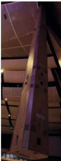
One of the two Fohhn columns that make up FOH
