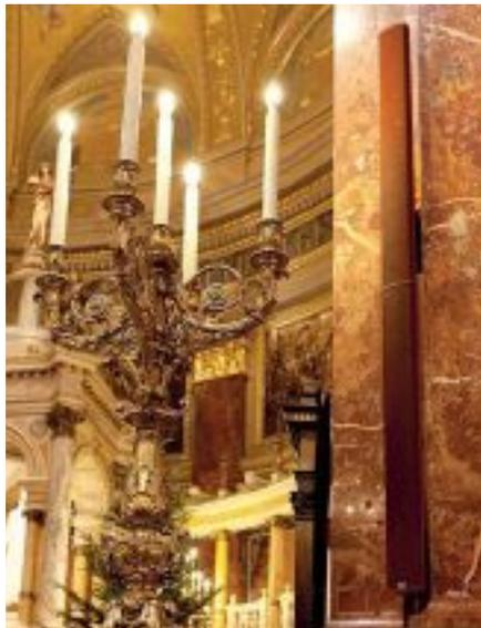
Column speakers can be easily hidden, as with these Pan Beam speakers in Budapest
