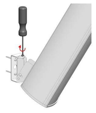
To adjust the vertical orientation of the speaker, loosen the bolts on both sides of the WS-2, tilt the speaker as desired and tighten the bolts again.
