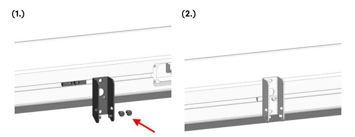
Horizontal speaker position: WS-2 housing plate should be positioned at the centre of gravity of the cabinet. For speaker longer than 1,3 m we recommend to use two WS-2 at a distance instead of one at the centre.
