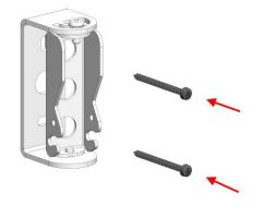
Mount the wall part of the WS-2 to the wall. Make sure all screws and dowels as well as the wall itself are suitable to carry the weight of the speaker. (Screw diameter max. 5 mm)
