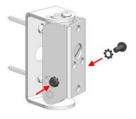
Guide the bolts of the housing plate into the hingeslots of the wall part. If suitable, you may insert e.g. a screwdriver into one of the threaded holes to join the two parts temporarily. (Picture shown without speaker) Assemble the parts with a tooth lock washer and an Allen bolt on each side. (Picture shown without speaker)
