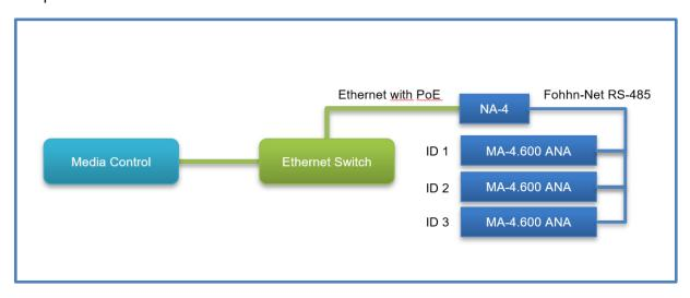
Some devices have an integrated Ethernet interface for audio, but still require an external Ethernet adapter for control:
