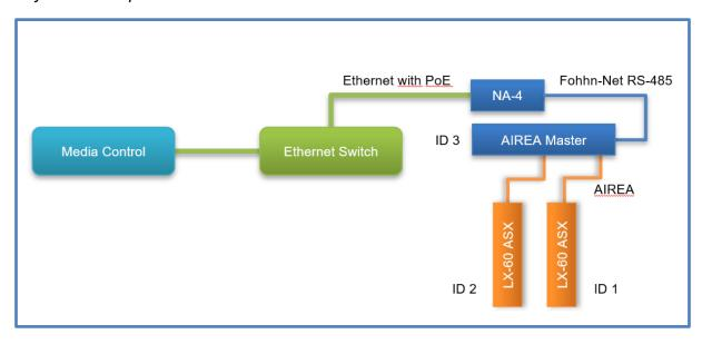
Units with their own power supply and AIREA input do not necessarily need an AIREA master; they can also be controlled via the AIREA output of an **ABX-5** or **ABX-6** and supplied with an audio signal at the same time.
