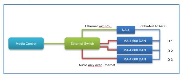
Try to keep the RS-485 sections as small as possible and use multiple NA-4s whenever feasible.
