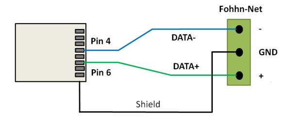
Pins 4+5 are assigned with Data- and pins 3+6 are assigned with Data+. Since the pins are simply connected in parallel, it is sufficient to use only pin 4 for Data- and pin 6 for Data+. The pins can also be combined, see the image below:
