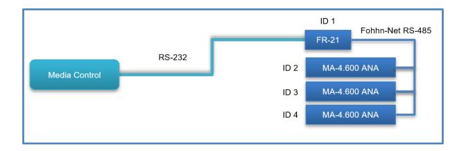
Only Fohhn devices with an RS-485-based Fohhn-Net interface can be controlled via the **FR-21**.
