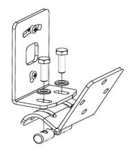
For mounting positions in the left-hand column of page 1, assemble the parts as shown above. Do not tighten the screws completely yet.
