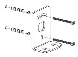
Mount the wall plate to the wall using suitable screws and dowels. (Screw diameter max. 5 mm)
