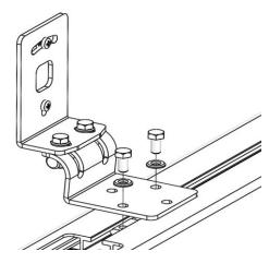
Position the housing plate at the centre of gravity of the cabinet. For speakers longer than 1.3 m we recommend using two WS-4 at a distance.
