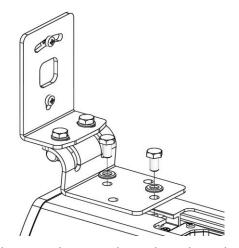
Position the housing plate anywhere along the T-slot of the cabinet. The slot nuts are supplied with the speaker.
