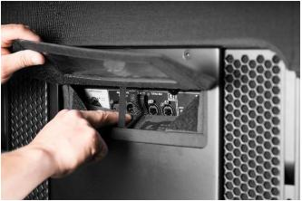
5. Tilt the lid outwards then connect the hook and loop fasteners on each side.
