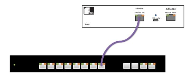
If there's no PoE Ethernet Switch available a PoE injector may be used (IEEE 802.3af compatible) or a standard USB power supply (5V, 500mA).
