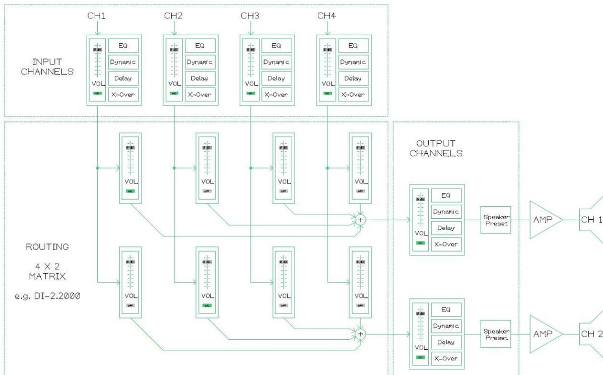
**Fig. 2: Four input channels are mixed to two output channels.
