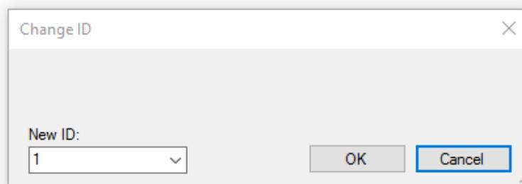
You can also change the ID of a **FOHNN** amplifier at any time while it is in use. To do this, the system must be in the **FOHNN-NET**. Proceed as follows:
