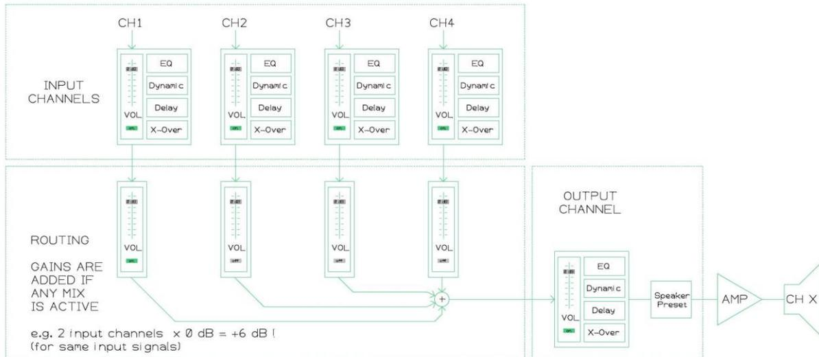
**Fig. 1: Four input channels are mixed to one output channel.
