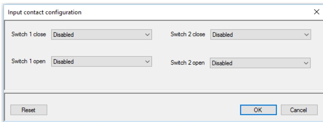
5. Select a setting from the drop-down menus for the “close” (*Switch 1/2 close*) and “open” (*Switch 1/2 open*) status: for example, you can deactivate the current status (*Disabled*) or load one of up to 100 presets (*Load Preset*).
