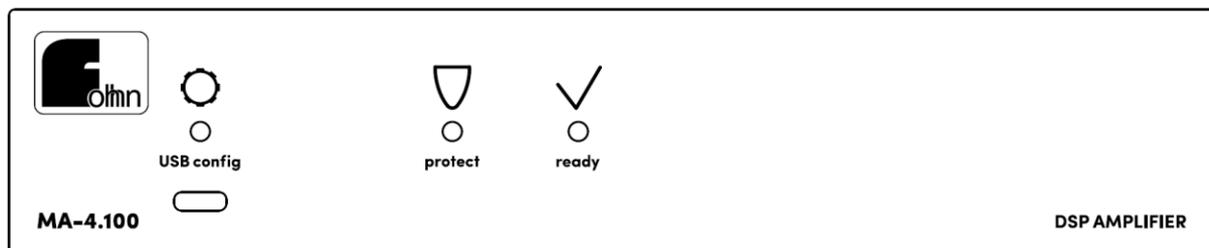
Status LEDs for a 4-channel amplifier
