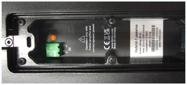
Cables should only be connected when the system is shut off.
