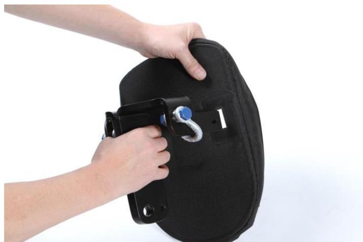
2. Connect the VFM-1 to the Focus Modular as described in section 3.2.5. The VFM-1 must be completely flush with the Focus Modular system's rain cover to guarantee impermeability. Turn the rain cover lid's protruding collar upwards.
