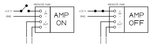
Switch states for 12 V control voltage
