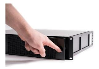
2. The filter foam that is to be cleaned can be found in the front panel's fan filter holder. Remove this filter foam and clean it, e.g. by blowing on it.
