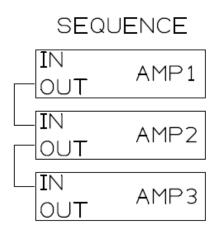
If the supply voltage for all three amplifiers is simultaneously and centrally switched on, amplifier 1 will delay the switch-on of amplifier 2. Amplifier 2 will, in turn, delay the switch-on of amplifier 3 etc.
