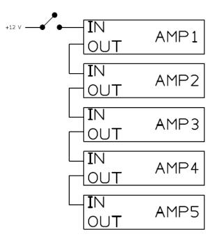
**Example 3:** Remote switch-on / switch-off of part of the stack while devices are connected with mains
