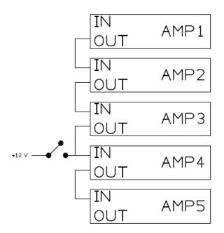
**Example 4:** Logical operation: Amplifiers 4 and 5 are switched on at the same time as amplifiers 1 to 3, but have a separate switch-off option.
