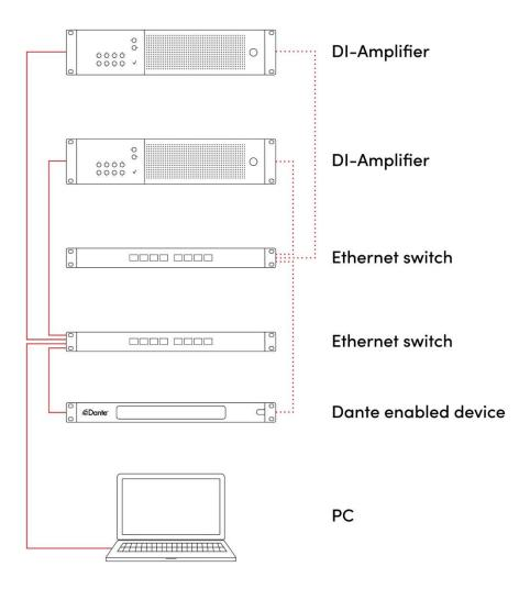
Example: Control of DI-Series amplifiers via computer and Ethernet switch using redundant cabling. (Here, all devices must be in "Redundant Mode".)
