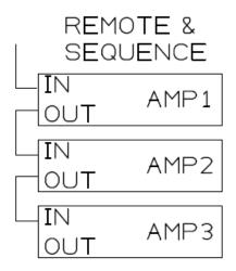
If a control voltage is not present at the *remote pwr in* of amplifier 1, all amplifiers will switch on one after the other. If a control voltage is present, all amplifiers will be/remain switched off.
