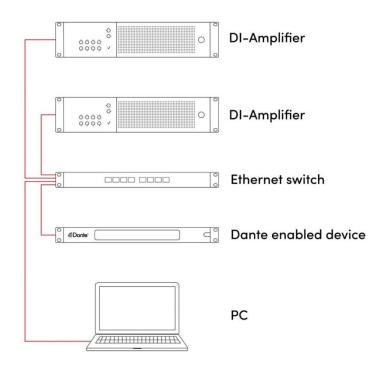
Example: Control of DI-Series amplifiers via computer and Ethernet switch using simple cabling.
