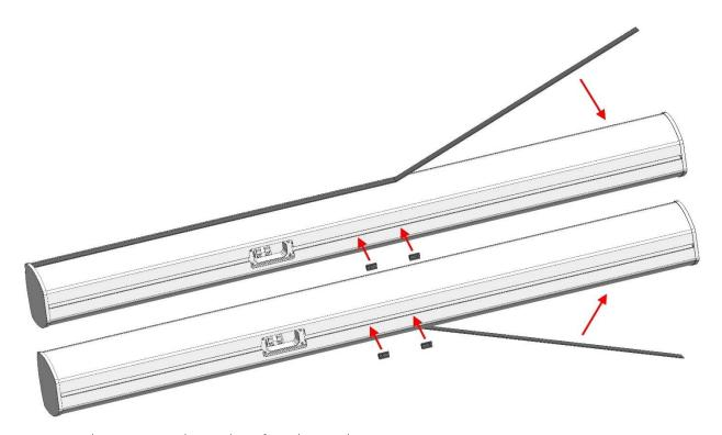
Insert two M6 slot nuts into the T-slot of each speaker. Attach the adhesive sealing tape to both enclosures as shown. Cut off the excess length.
