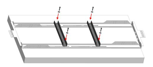
Place the VESA wall mount kit of the display on top of the VESA-Bracket-S/L and screw them together using Allen bolts and washers.
