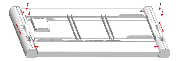
Push the speakers against the display and align them vertically. Bolt them to the VESA-Bracket-S/L using the slot nuts and M6 Allen bolts.
