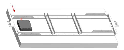
Attach a Fohhn system amplifier (e.g. MA-4.100) to the bracket. There are several possible positions left and right.
