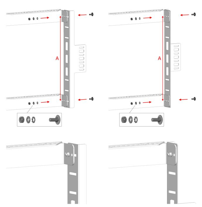
Arrange the six bracket parts according to the images in 1. or 2. If depth of display is smaller than or equal to 90 mm, refer to image 1., otherwise to image 2. Choose dimension "A" according to your display's VESA standard (200, 300 or 400 mm). Screw the parts together using carriage bolt, tooth lock washer, washer and nut.
