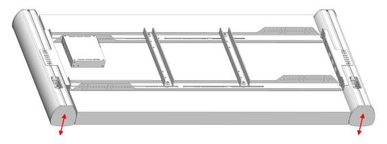
If desired, align the speakers in depth to level with the display's screen. Please refer to 1. or 2. Make sure all screws and nuts are tightend correctly.
