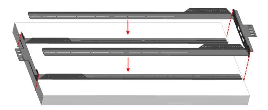
Put the VESA-Bracket-S/L against the rear of your display and align it with the display's outer edge as shown.
